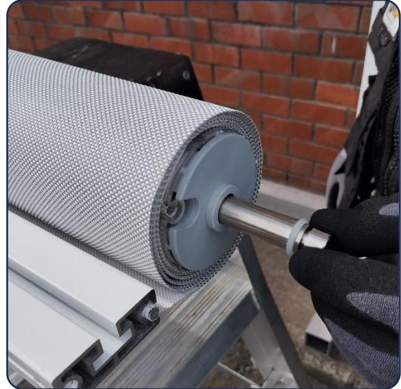
Inserting Idler pin and cap into the opposite end of the blind
